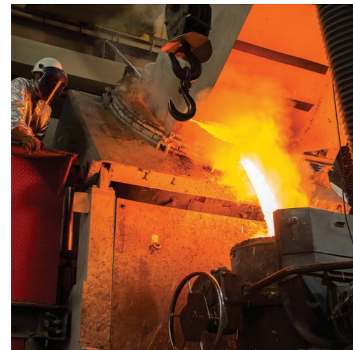
Standard bronze pour from furnace to ladle in our FLSmidth foundry for EXCEL parts
